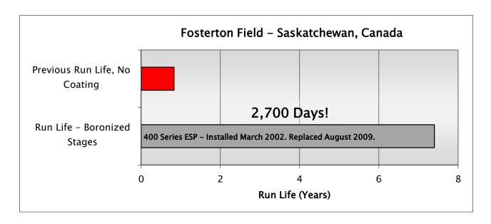
In the Fosterton area, typical run life of an ESP is up to one year. At which point there is significant wear due to abrasion on the ESP Impellers and Diffusers, causing them to be replaced.
