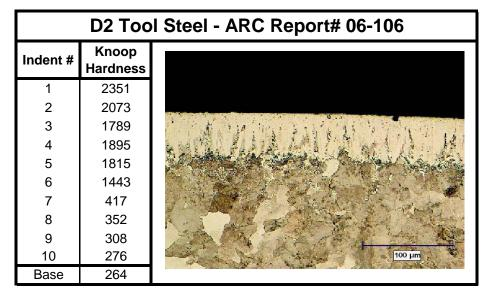
The Knoop microhardness testing was conducted using a 25g load. The first indent was approximately 10 micron below the surface, with subsequent indents at 0.0005" intervals, spaced within guidelines suggested by ASTM standard C1326-99.
