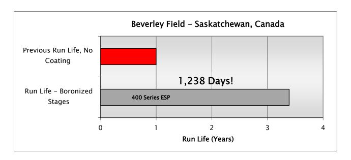
In the Beverley Oil Field area, typical run life of an ESP is up to one year. At which point there is significant wear due to abrasion on the ESP Impellers and Diffusers, causing them to be replaced.
