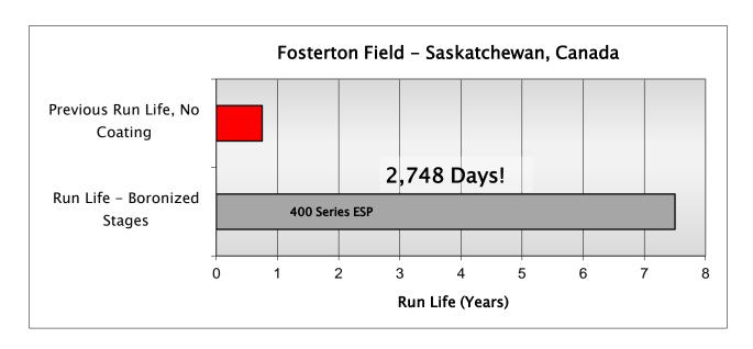
In the Fosterton area, typical run life of an ESP is up to one year. At which point there is significant wear due to abrasion on the ESP Impellers and Diffusers, causing them to be replaced.
