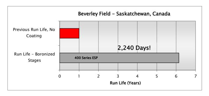
In the Beverley Oil Field area, typical run life of an ESP is up to one year. At which point there is significant wear due to abrasion on the ESP Impellers and Diffusers, causing them to be replaced.
